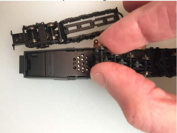
**Step 7:** Install the traction-tired driver (just push in).
