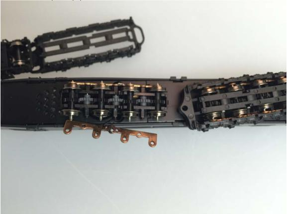
**Step 6:** Pull the rear-most driver up and out of the gearbox.
