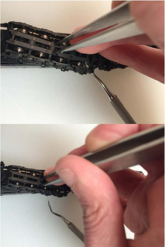
**Step 5:** Remove the pickup plates.
