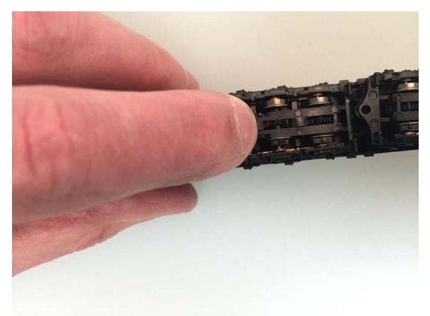
**Step 10:** Re-align the trucks and insert the swivel pin.
