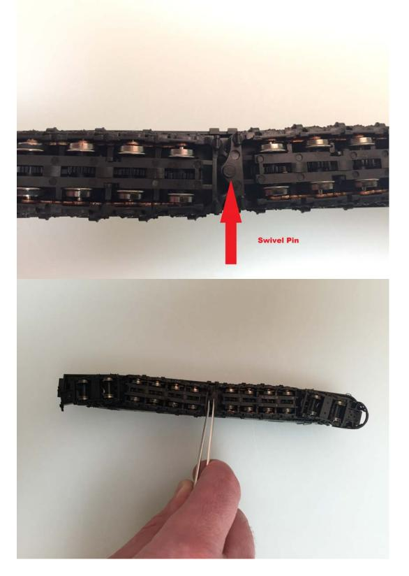
**Step 2:** Swivel the trucks so that they can be separated as shown in the photo.
